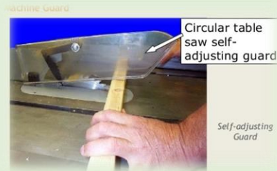
Self-adjusting guards, Fig. 5
